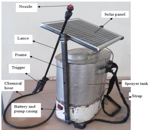
Figure 1: Pictorial representation of the developed solar powered sprayer
