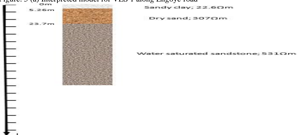
Figure 5 (b) Geoelectric and inferred geologic sections for VES 1 along Engoye road
