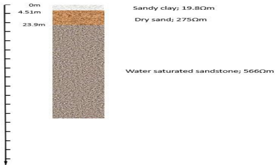
Figure 7 (b) Geoelectric and inferred geologic sections for VES 4 along Beeh Hostel road
