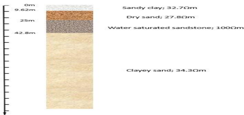
Figure 8 (b) Geoelectric and inferred geologic sections for VES 3 at Otuoke market.
