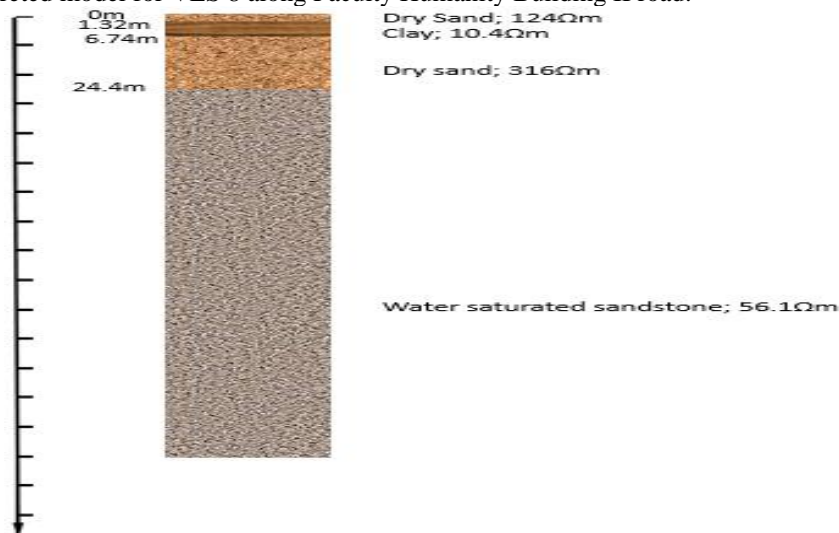
Figure 9 (b) Geoelectric and inferred geologic sections for VES 8 along Faculty Humanity Building II road In summary of the interpreted results, eight VES stations displayed three-layered geoelectric sections while nine VES stations are four layered geoelectric sections.
