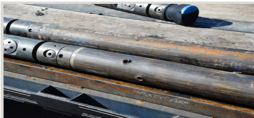
Figure 1: A perforating gun for creating pathways in the casing for the fluid injection during the hydraulic fracturing treatment of a well. (Source: U.S. Geological Survey, 2016)
