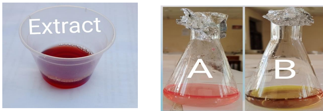
Figure 5.0: Ethanolic extract of red onion peels, Colour Changes in acidic solution (A) and basic solutions (B)
