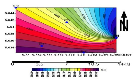
Figure 10: Sand-I Top Sand-M: The contour interval across sand-I is 10 ft (3.048 m). There is an increased in elevation from South to the North in ET-1. In ET-3, there is a
